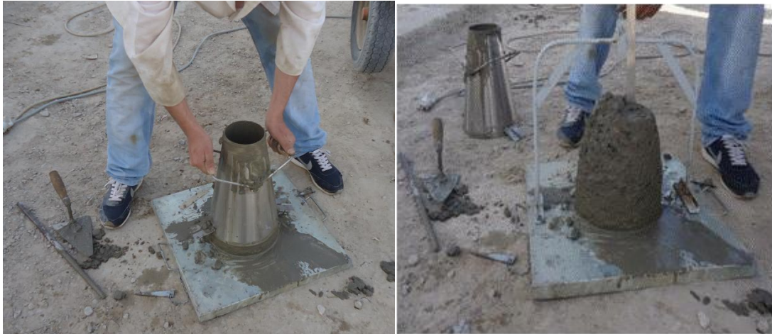
Figure 5. Workability test of studied concrete.
